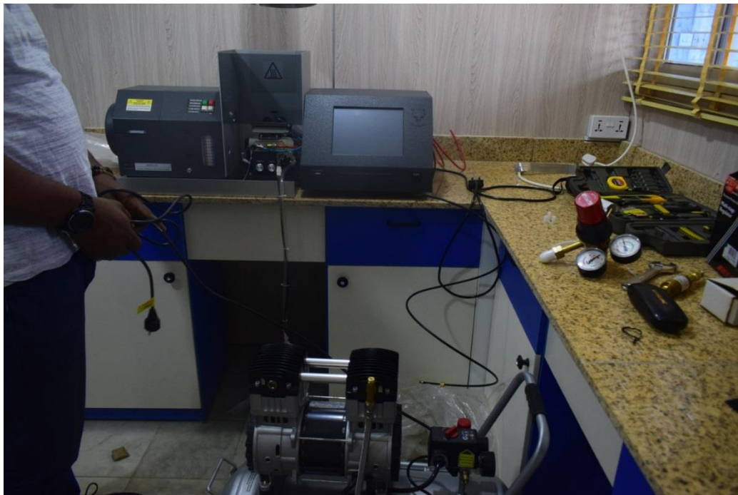
Installation of Atomic Absorption Spectrophotometer (AAS) and other components at NIHSA Laboratory, Headquarters Abuja
